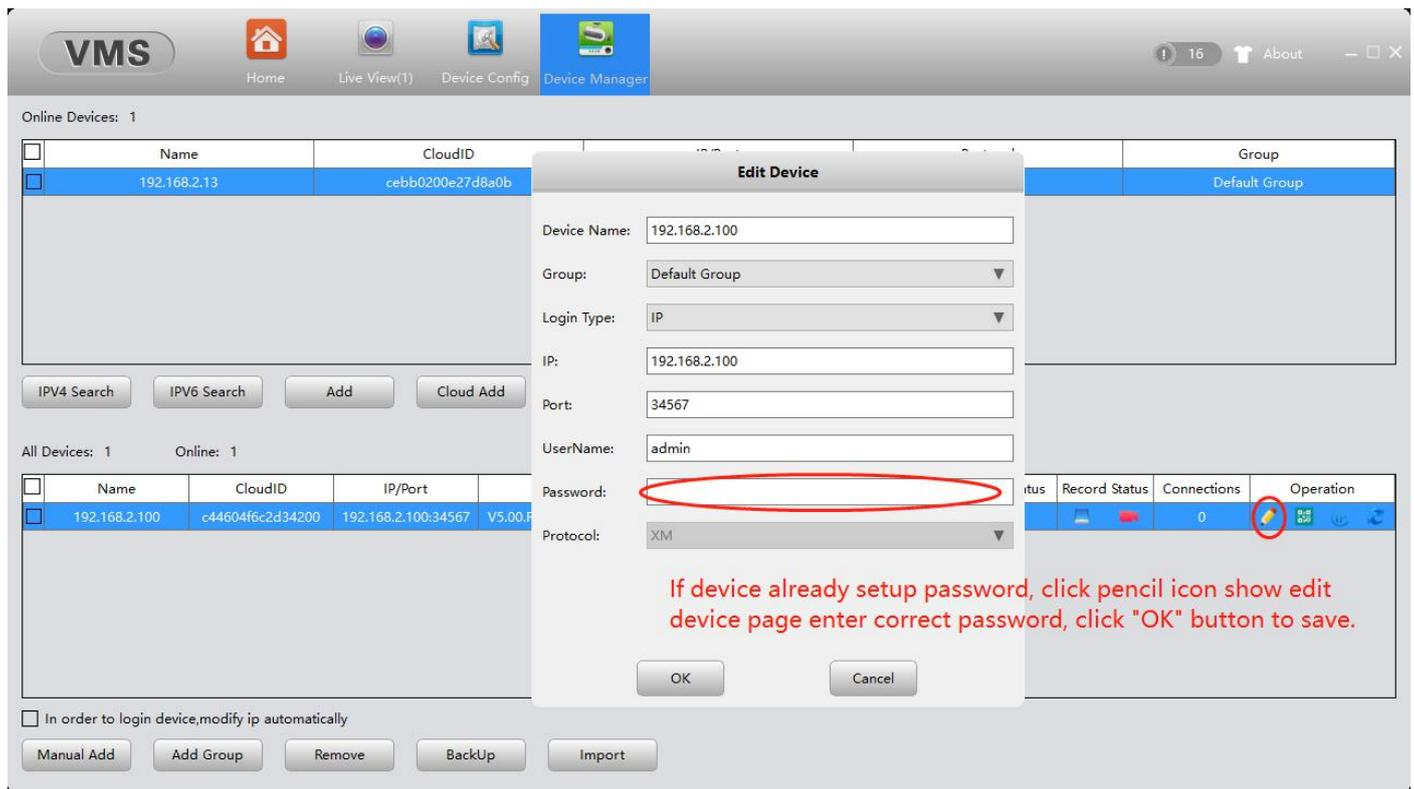
Add remote device. Click "Cloud ID" button, input 'Device Name' 'Cloud ID' and 'password'(default null password), then click "OK" to save and exit.
